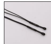
Lead type thermistor JAXA Qualification 2016
